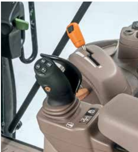
AutoPowr on the right-hand console
