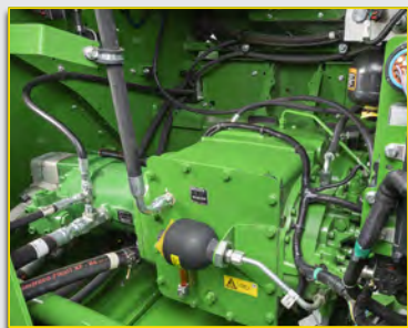
A. Clean transmission, hydraulic valve block, and front axle area.
