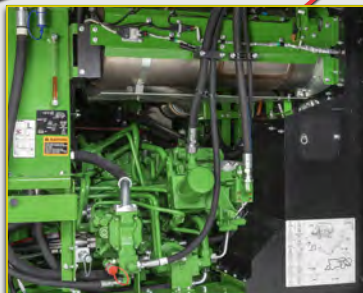
C. Clean door latch, auxiliary drive gear case, hydraulic pumps, and exhaust components.
