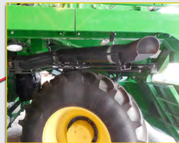
E. Clean exhaust system components, including heat shields and hanger brackets.
