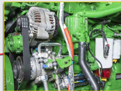
E. Clean the alternators and check the engine belts and pulleys.
