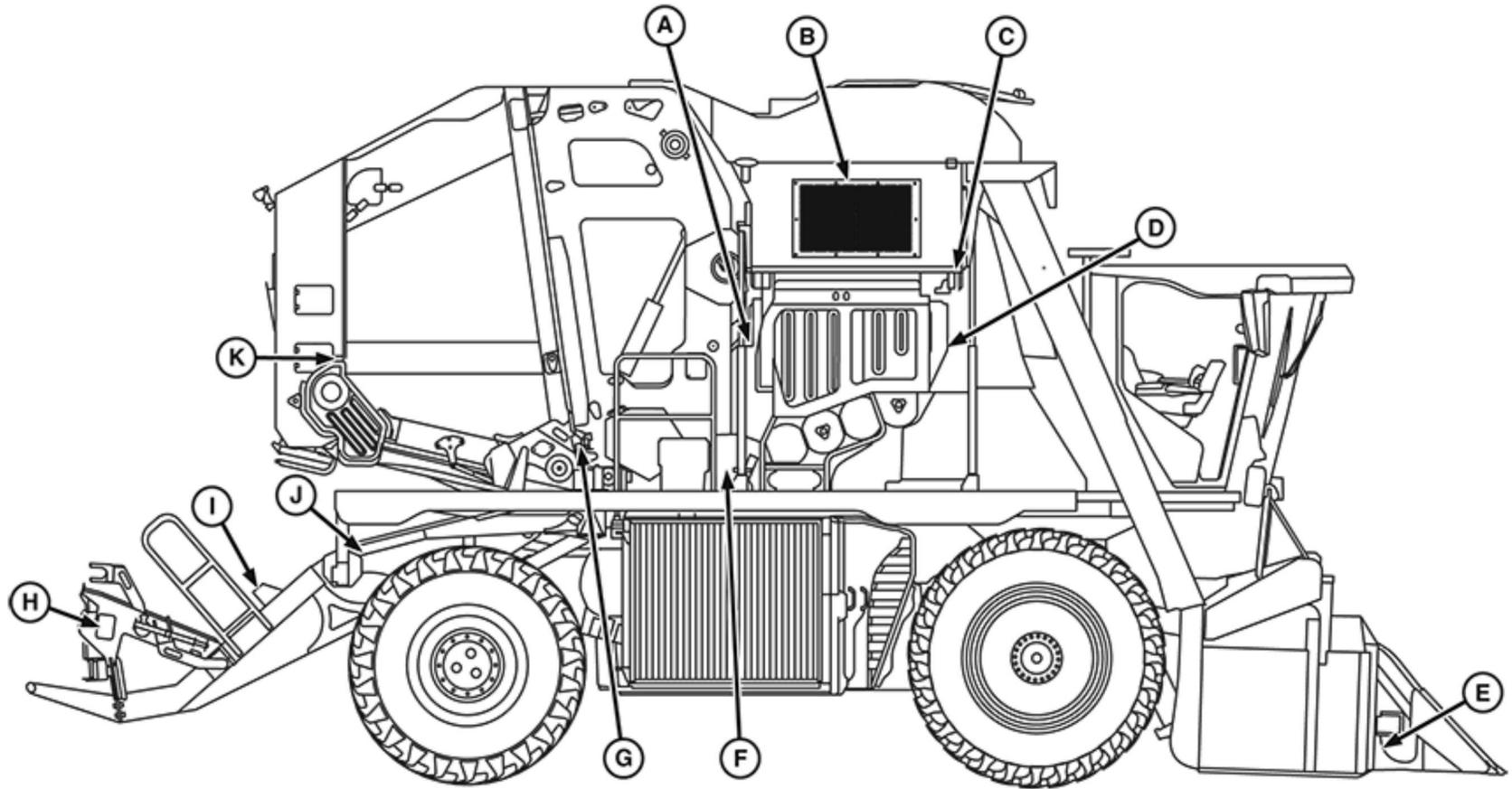
A - Lower Accumulator Sensor (receiver)
