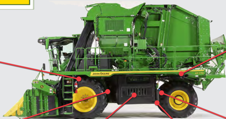
A. Clean transmission, hydraulic valve block, and front axle area.
